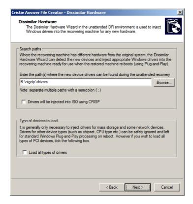
Tick **Drivers will be injected into ISO using CRISP** if you intend to manually add extra DHW drivers to your customised boot ISO during the CRISP ISO generation phase. This can be in addition to any drivers contained on the driver path specified above.
