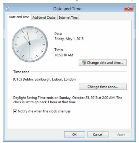
Note: the Additional Clocks and Internet Time tabs are operational. In fact it is possible to synchronise the system time with an NTP time server if required.
