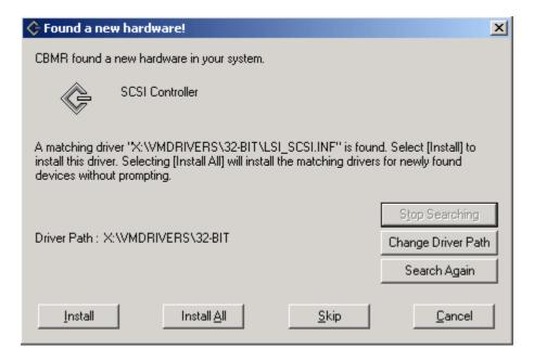
If you are satisfied that the found driver path is correct, click on <a href="Install">Install</a> and the driver will be installed. The device scan will continue and may find, for example, other mass storage or network devices. Follow the steps above to install.
