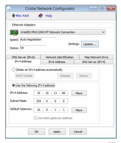
Set the new IP address, subnet mask and gateway IP address. The More button will allow the system to have more than one static IP address. Click on Apply to confirm the settings for the selected adapter.
