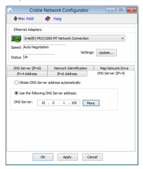
Select the 'Use the following DNS Server address' radio button and enter the new DNS IP server address. If required, select the More button to add several DNS IP addresses. Press Apply to activate the new address.
